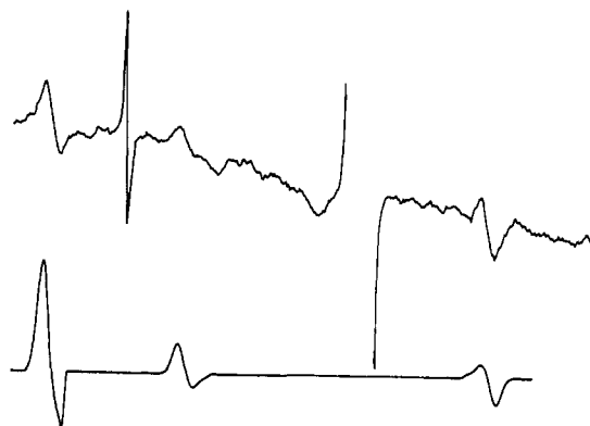
Figure 7. Simulation of the \Delta M_s = 1 and \Delta M_s = 2 regions of the ESR spectrum from 1000–5000 G of dinitrene 3 . Curve a is experimental; curve b is simulated using |D/hc| = 0.189 \text{ cm}^{-1} , |E/hc| = 0.00 \text{ cm}^{-1} , and g_{\text{iso}} = 2.003 .
